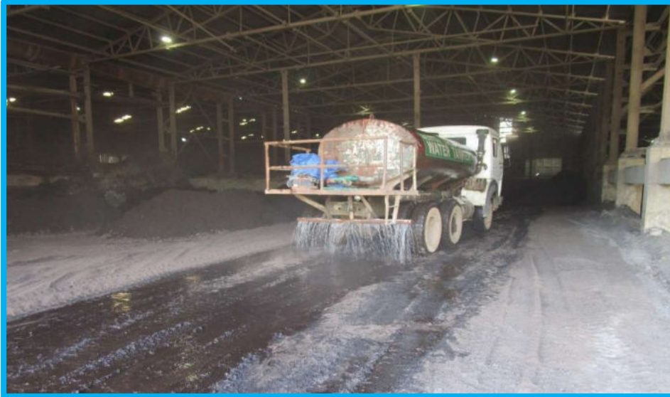
Water Sprinkling through Water Tanker Inside the coal storage sheds
