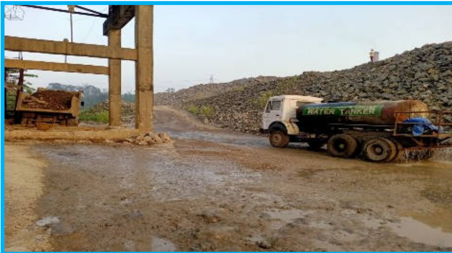
Water Sprinkling through Water Tanker In all internal Roads at Plant
